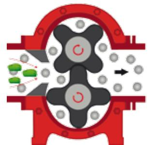
**Injection A:** Asymmetrical pump housing segments with the InjectionSystem design, arranged on the suction side
