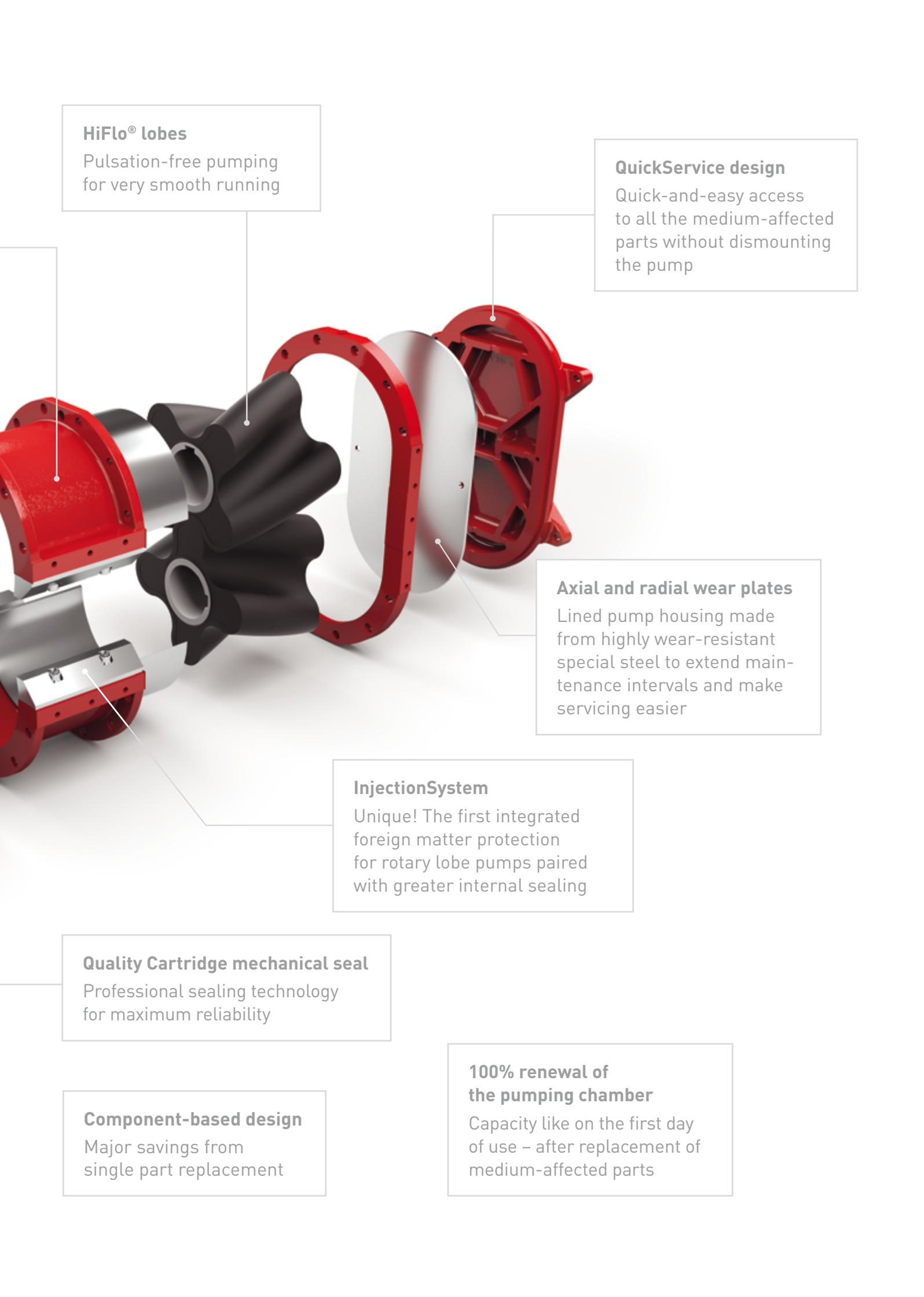
The image shows an exploded view of a rotary lobe pump assembly. The main components are: two black lobes, a red housing with a silver lining, a silver axial wear plate, a red radial wear plate, and a red injection system. The assembly is shown in a disassembled state to highlight individual parts.
