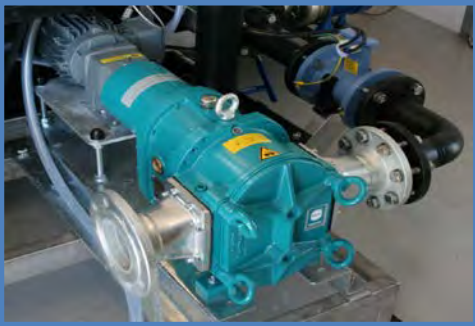
Biomass is introduced to the machine by variable drive pump, and flowmeter for control and documentation.
