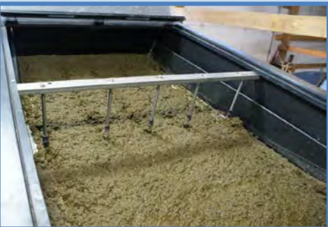
Gentle process is used by gravity to separate water from solids.
